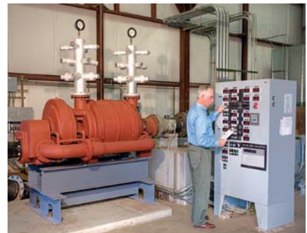
A Vooner FloGard high-vacuum two-stage pump being tested
